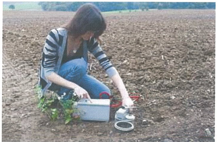
A portable soil respiration system measuring soil CO 2 flux
